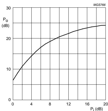
Fig.4 Output power as a function of input power.
